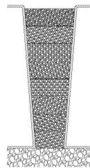
Fill Cones in 6" layers from the bottom up, compact each layer. Use recommended backfill material.
